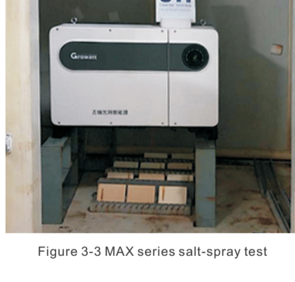
Figure 3-3 MAX series salt-spray test
